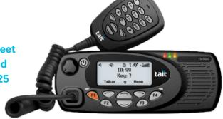
The TM9400 is capable of AES encryption, Over-the-air Rekeying (OTAR), various emergency modes and is IP54 rated to keep those relying on the mobiles safe and efficient. The TM9400 also has an options slot allowing extension of capabilities and a range of remote mounting and control head options.
