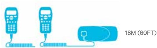
Dual Control Heads can be used to control a mobile radio from two different locations – for example, this could be the front and rear of a vehicle, or two different desks in an office dispatch situation.
