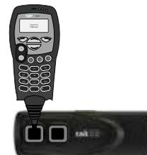
**Note 1:** The dual-head upgrade kit provides one complete remote head, one remote control head interface which is fitted to an existing local control head and one control head interface box.
