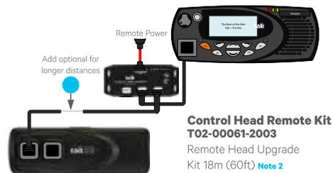
A remote cable of up to 20ft (6m) is allowed between the radio body and the remote control head
