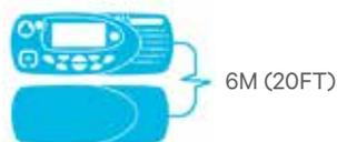
Tait provides a range of Control Head Remote Kits in 3 cable lengths – 6m, 12m, or 18m. These kits include all the components you will need to remotely mount the radio body and control head of your Tait Mobile Radio.
