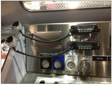
On Display in Dauphin: Fort Garry Fire Trucks pumper outfitted with two Motorola XTL 2500 dual-head radios supplied by Alcom. One radio for on-scene and one for wide-area communications.
